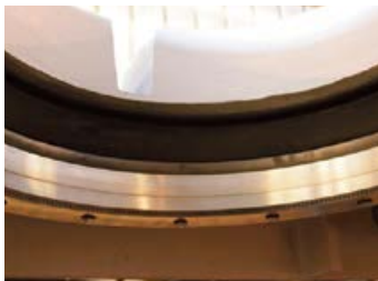
Graphite Ring installed in a billet casting mold
