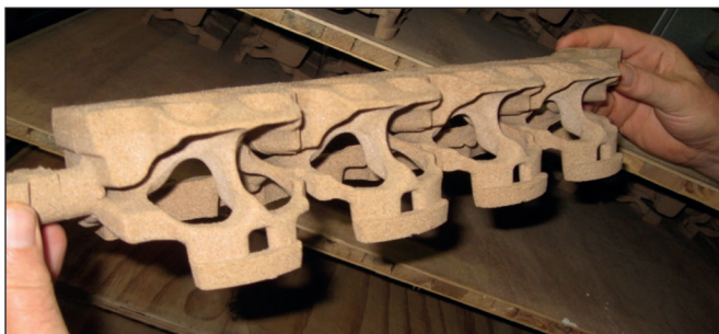
Figure 2. A complicated core design for an automotive casting made in South Africa.
